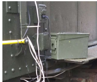
Gift Shop – Plug in AC cable on North end of Gift Shop car. RPO – Works with gift shop
